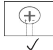
Insert bolt when connecting piece direction is properly lined up.
