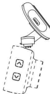
1. Place the GPS module together with the camera holder as shown in the picture above. The GPS module fastens to the holder with the help of the magnets. The shining of the LED diode GPS (14) shows that the GPS module has been fastened correctly – this is also the case when the holder is connected to a power source.
