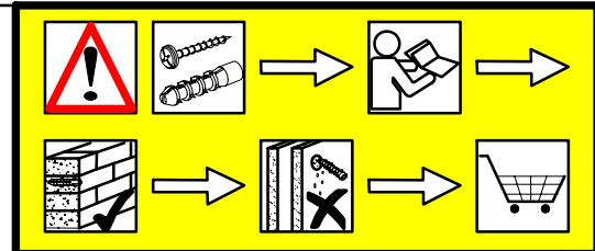
Caution! The wall must be examined before assembly. The included universal wall plugs are only suitable for use in solid masonry such as concrete block or brick. Do not use the wall plugs on hollow brick, lightweight block, surfaces such as gypsum plasterboard or other framing systems. If applicable, specific wall plugs must be used! These are available at a specialised store (hardware store). In case of non-compliance, the manufacturer/importer does not assume liability.
